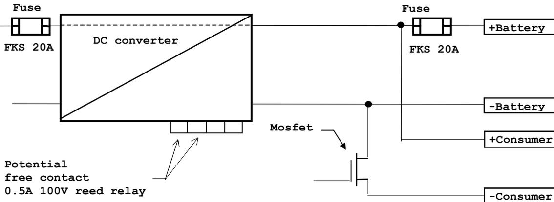
If the accu voltage will be smaller than 11.3V/22.6V for ca. 60 sec., a reed contact will be activated. In this way a diesel generator can be controlled.
