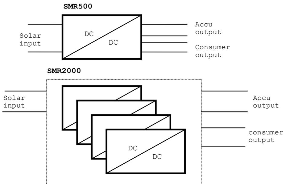
⇒ The micro controller system consists of buck converters being regulated to maintain the optimal solar voltage while temperature and solar radiance changes. (Powertracking). It is about 16–18V in a 36 cells solar modul and a temperature of 20°C. This results in winter in an average increase of charging current of 15%.
