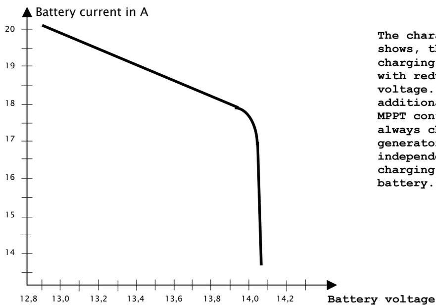
The characteristic curve shows, that the battery charging current increases with reducing battery voltage. This is an additional advantage of the MPPT controller, which always charges the maximum generator current independently of the charging condition of the battery.
